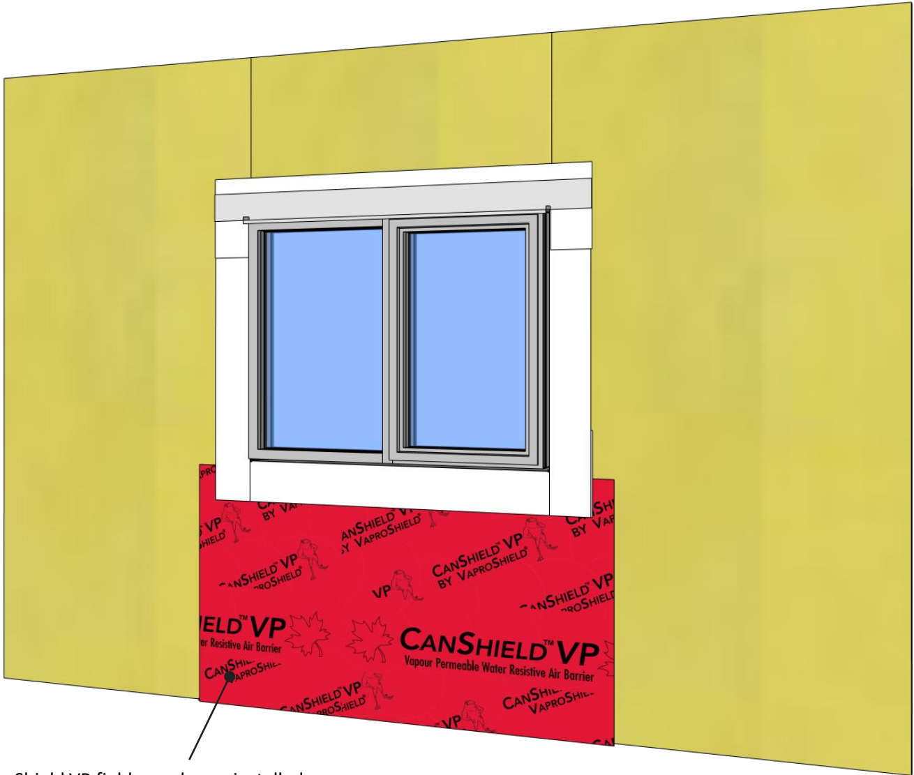
CanShield VP field membrane installed underneath 6" flap of VaproFlashing SA to create shingle effect
